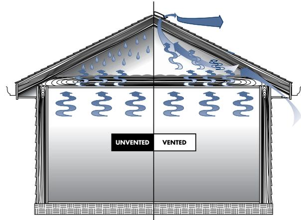
Unvented: Moisture rising up through the house condenses in the attic, causing damage to studs, insulation, and other materials.
