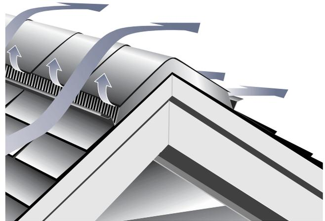
An externally baffled vent "pulls" air from the attic from both sides of the ridge vent.
