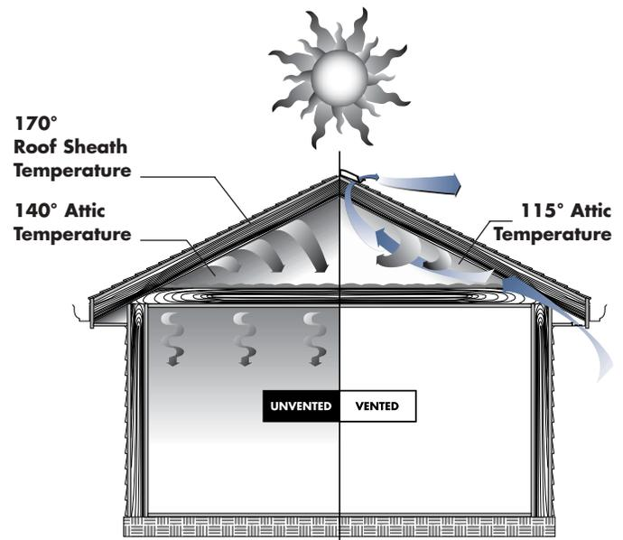
Unvented: Radiant heat penetrating through roof sheath and attic enters living areas of home.
