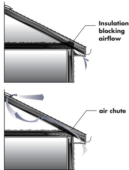
(Top) Insulation blocks undereave intake vents preventing proper airflow into the attic.
