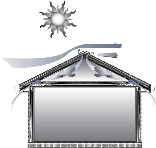
Thermal Flow (effect whereby cooler air falls, warmer air rises) and Natural Flow (effect due to wind) come together to ventilate an attic.
