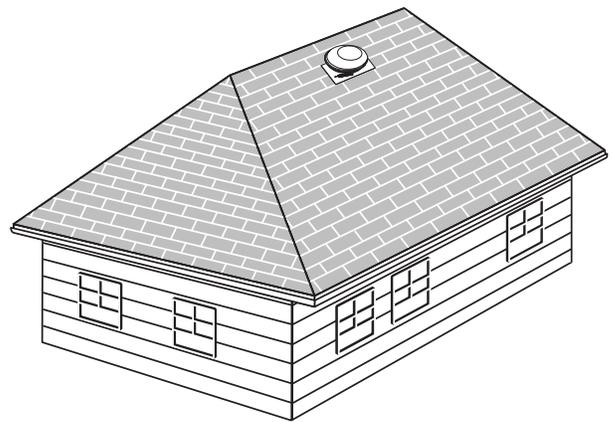
Power fans are used to move large volumes of air – a good option for hard-to-vent hip roofs that have limited horizontal ridge length available for ridge venting.
